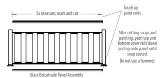
Mark and cut top and bottom lengths, inside to inside posts, minus 1/16" clearance.
